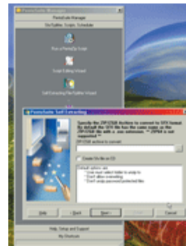
The PentaSuite manager allows you to select one of the many programs included with the PentaSuite program. In this case we have selected the "Self Extraction Wizard" which allows you to compress groups of files into *.exe program. This program will automatically open and extract all the files when started.
