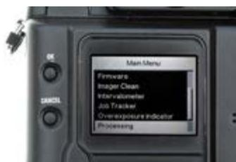
This is the elusive ERI menu on the Kodak DCS 720x. Pressing this will advance you to the menu that controls how files are saved and automatically deleted.
