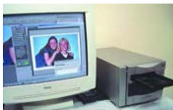
Nikon 8000ED film scanner with film holder inserted and setup menu on monitor.
