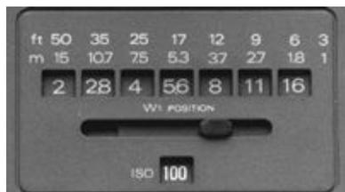
The exposure calculator on manual flash units (and on auto units when used in manual mode) tells you what aperture to use when shooting at a given flash-to-subject distance, once you've set the ISO speed of the film you're using. Note that the farther away you are, the larger the aperture required. At great shooting distances, the flash can't produce enough light to provide proper exposure even with the lens wide open.
