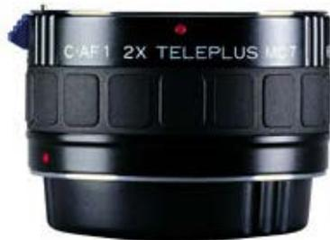
Tele-converters, like extension tubes, fit between the camera body and lens. But unlike extension tubes, converters do contain glass elements. Tele-converters increase the focal length of the camera lens, while retaining its original minimum focusing distance, thus providing greater magnification ideal for close-up work
