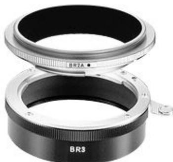
A lens-reversing ring lets you mount the lens on the camera "backwards"—with the mount end out. With normal and wide-angle camera lenses, this results in greater magnification and sharper images, especially at the edges. Just attach the reversing ring to the camera, then screw the lens front-first into the reversing ring.
