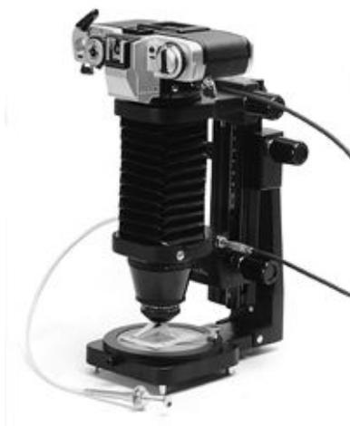
A very useful bellows accessory is a macro stand, which holds both camera and subject in position for sharp, precise close-up images. Special bellows lenses, such as the one shown here, can yield magnifications up to 25X with the bellows unit.
