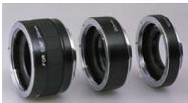
Extension tubes are just spacers that fit between the camera body and the lens. They increase the distance between the optical center of the lens and the film, allowing you to focus closer and thus increasing magnification. The longer the extension tube (or the shorter the camera lens), the greater the magnification. You can combine extension tubes to increase magnification.
