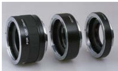
Extension tubes are just precise spacers that fit between camera body and lens. They increase the distance between the optical center of the lens and the film plane, thus producing closer focusing and greater magnification.
