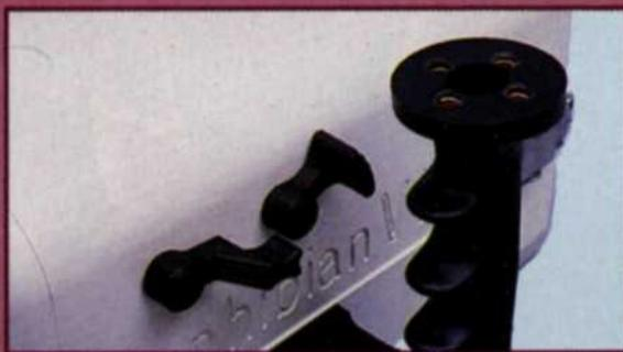
The Amphibian V11 housing weighs only 15.5 pounds with the camcorder inside. By calculating this weight versus housing displacement, Amphibico has eliminated the need for bulky lead ballast. The system is a few ounces negative, balanced to avoid the need for wings. The controls operate electronically, eliminating levers or rods.
