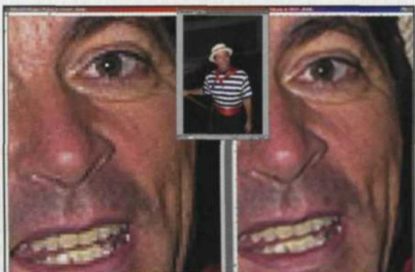
Nikon D1 image that had been reduced for Web page. File was saved as Fractals and reopened at a 400% enlargement on the right. Notice the reduction of the jaggies in both the eyes and the teeth.
