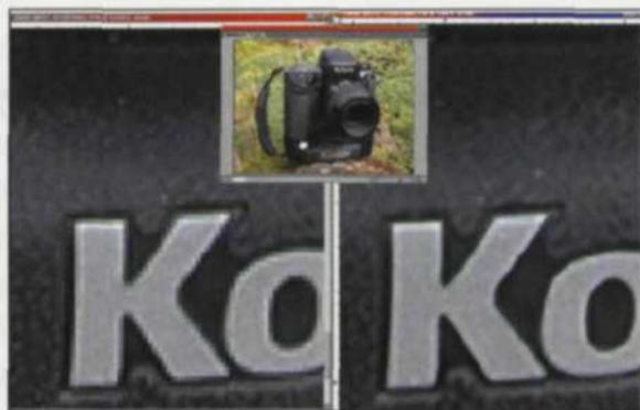
Digital image shot of Kodak digital camera. Original file had been reduced to less than 900 pixels on longest side for transmission on the Internet. File was saved as an .stn file and reopened at a larger size with a dramatic reduction in pixels in the Kodak lettering. JPEG on left and Fractals on right.
