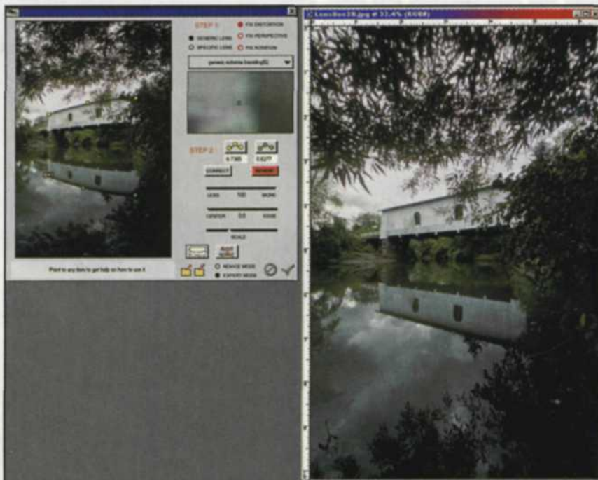
LensDoc filter can correct for pincushion and barrel distortion created by various lenses.
