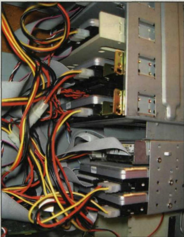
RAID drives can be in an external box, or inside the computer that it is attached to. This is a typical setup with the RAID inside the computer. An extra cooling fan was installed to keep the heat down.
