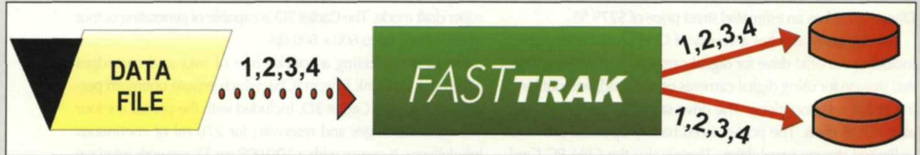
RAID 1 or mirroring configuration. The data is saved twice on two drives. If one side fails, the other can rebuild a new drive.
