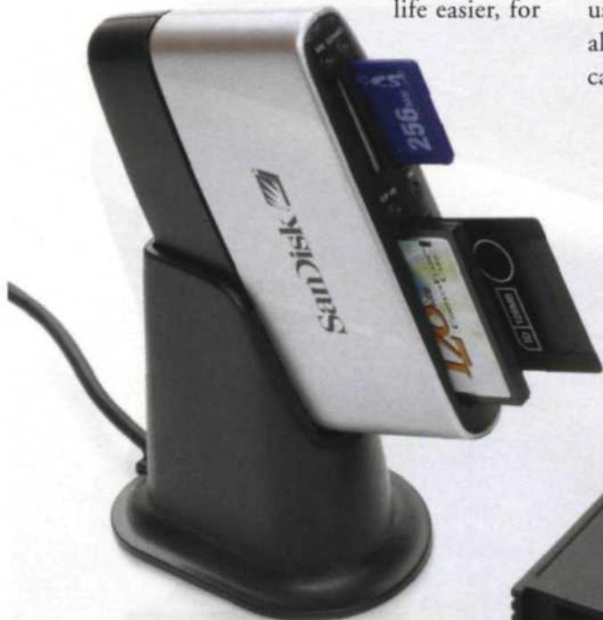
A memory card reader provides a simple means of transferring digital images from camera to computer.
