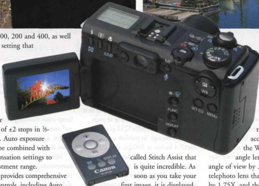
The LCD panel on the back of the G5 swings and swivels to aid composition when shooting from odd camera angles.
