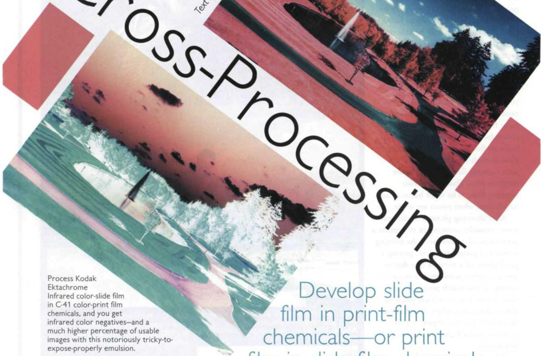
Process Kodak Ektachrome Infrared color-slide film in C-41 color-print film chemicals, and you get infrared color negatives—and a much higher percentage of usable images with this notoriously tricky-to-expose-properly emulsion.
