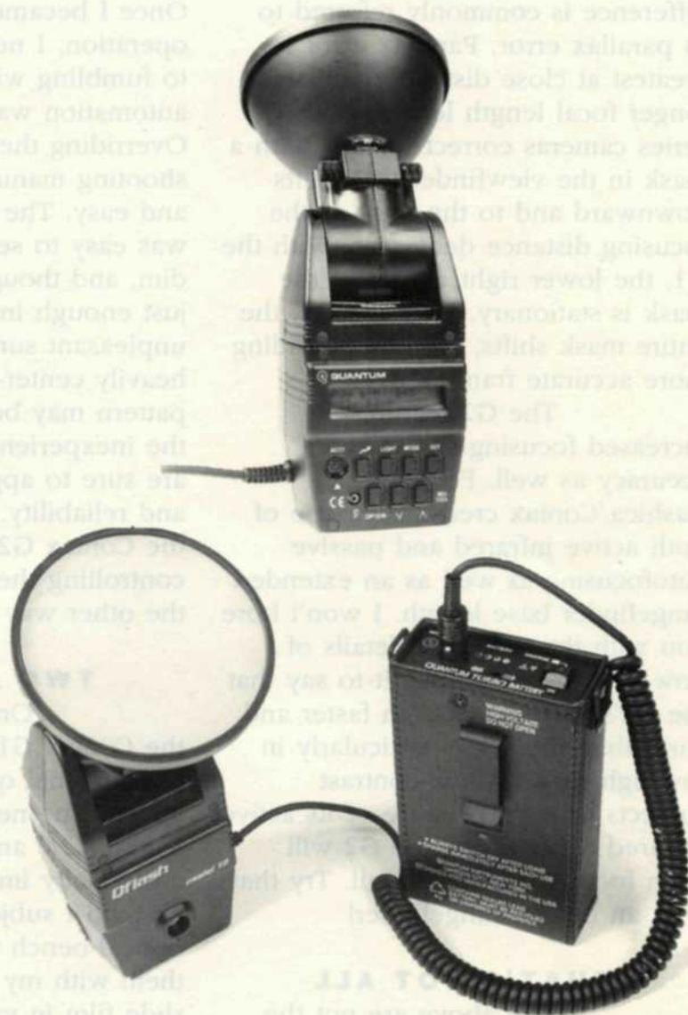
The base of the Qflash has an LCD display panel that provides a variety of information about setting up your flash and monitoring its functions. The first row of buttons includes the flash-fire, light, mode, and set functions. The mode button sets the flash up for manual, auto, TTL, or stroboscopic operation. Once you have selected a mode, you can then fine-tune your selection with the up/down or set buttons.
